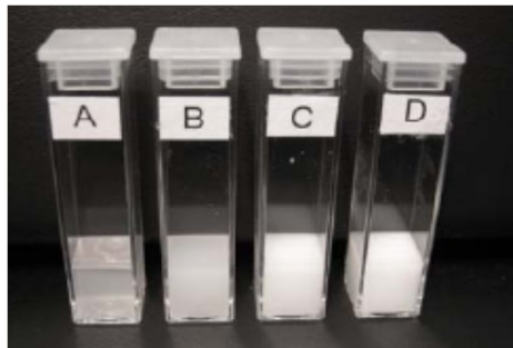
Figure 2: Photograph of cuvettes containing various concentration of the \text{TiO}_2 dispersed in 10mM NaCl. A = 0.01% w/v, B = 0.1% w/v, C = 0.2% w/v and D = 0.3% w/v
